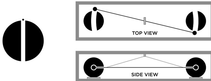
Fig. 2. – Left: Idealized (simplest) experimental method—sphere in outer space. Right: Practical experimental method—modified Cavendish balance in Earth-based laboratory.
